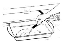
Unclip hose and allow defrost water to drain through the hose into a flat pan. After defrosting and cleaning, hook drain hose in place and replace the base grille and drain cap.
